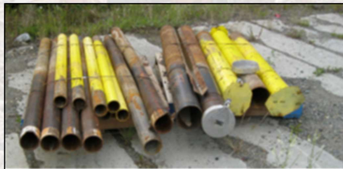
Steel casings and bollards decommissioned and staged for reuse at the USACE Bear Creek Remedial Action and Site Closure
