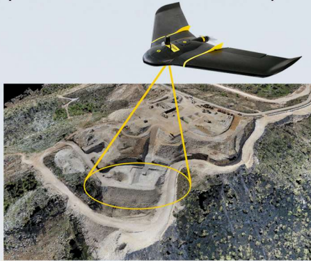
The image above is not a photograph, but a 3D rendering comprised of millions of data points from our drone surveying system. Below, UAV operators upload survey data.
