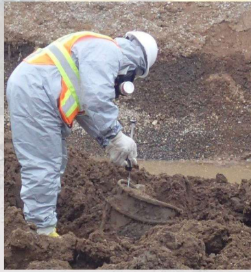
Sampling soil using X-Ray Fluorescence
